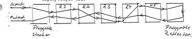
R1 and R5 stop each time befor encypherment R2 steps when R1 is notched and/or R2 is notched R3 steps when R2 is notched and/or R3 is notched R4 steps when R3 is notched.
