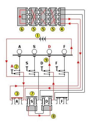
The schematic on the left shows the arrangement of the wheels and plugboard of the Enigma. For clarity only four of the 26 circuits are shown. A single cable is connected to the *Stecker* board between sockets D and S.
