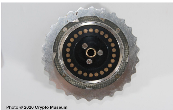
Figure 10. Enigma T wheel with five notches.
